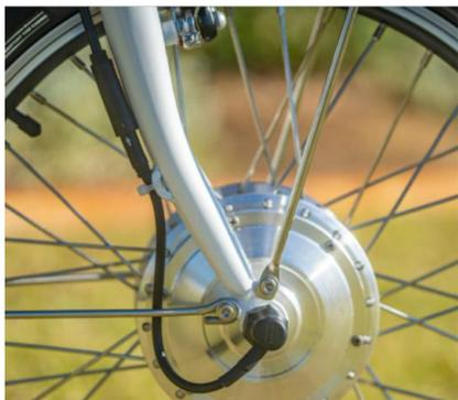
If you need to remove the front wheel, for example, to replace the front tyre, then the motor can be unplugged to aid disassembly. The plug is located on the right side of the forks as shown (below).
