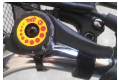
To release the tilt lock, push the lever forward (away from the rider). To lock the Tilting mechanism pull the lever in the opposite direction.
