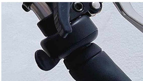
The throttle is available all the time the power is switched on at the left handlebar display. The throttle can be used whilst pedaling in any of the assist modes to give extra help as required. The throttle is not limited by the assistance level selected and is available to give up to maximum power at all times.
